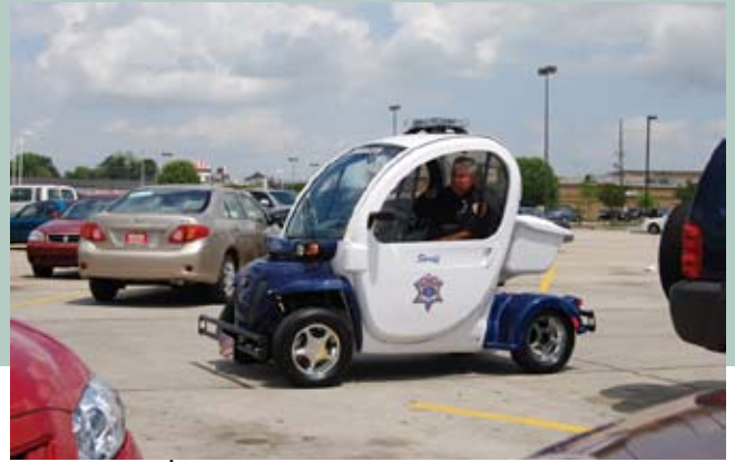
Deputy Elbridge Charlton patrols a parking lot in an electrically-powered vehicle. With a range of 30 miles on a single charge and a top speed of 25 MPH, the vehicles allow a deputy to cover much more ground than if he were working on foot.
